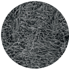
LongLife Felt Smaller fibres More pores Thicker media
